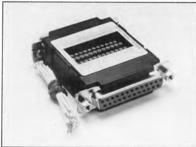
The patch box has male and female connectors, the connector pins being interconnected within the box by jumper leads. These are fitted with easy push-fit connectors, so that the pin-to-pin connections can be changed in seconds, and the
